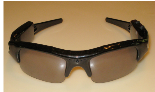
Figure 1: Low cost pinhole camera glasses. The camera is mounted on the nose bridge.
